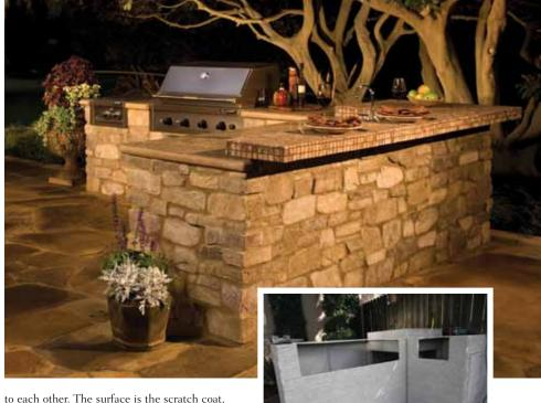
to each other. The surface is the scratch coat, meaning once the blocks are in place, brick, natural stone, or architectural stone veneer can be applied directly to the surface immediately. The entire process takes a fraction of the time used in traditional methods for creating such spaces.
